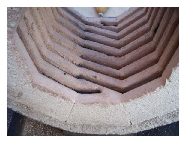
A close up of the brick face shows the grooves cut for the heating element. I painted the surface with a ceramic paint that provides a harder surface plus is highly reflective to the heat.
