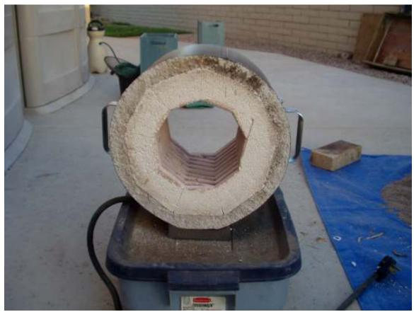
If you look into the body section, you will see that I used 9 firebricks. These are soft firebricks, which are a better insulator than hard bricks plus are extremely easy to cut. Between the firebricks and the outer skin is a layer of 2300 degree F castable refractory. It is 5 to 20% perlite and very delicate. It is also an excellent insulator.
